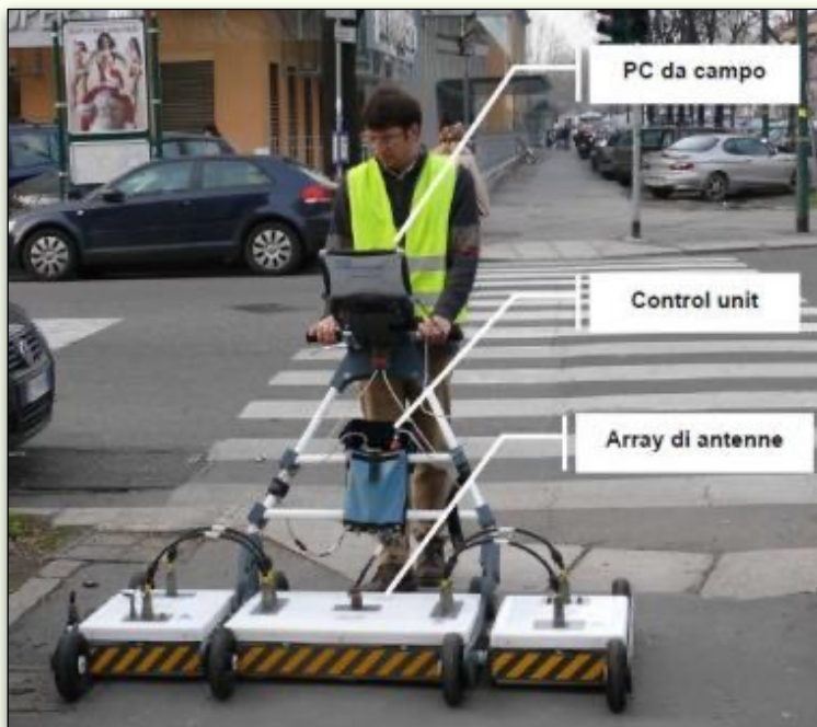
Figura 5 – Georadar ( Ground Penetrating Radar-GPR )
